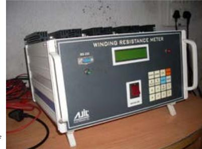
Introduction : These instruments are specially designed to measure the resistance of the inductive object such as transformers, inductors, coils and other windings. These instruments are widely used in the power and distribution transformer manufacturers, motor manufacturers etc.
